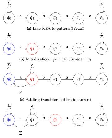
(d) Advancing current with character *b* to  $q_2$ , lps stays in  $q_0$  due to  $\Sigma$  transition.
