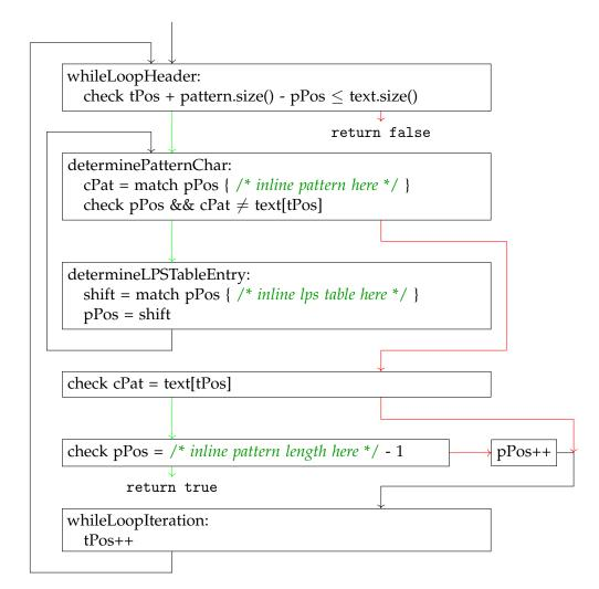
**Figure 3.1.:** General control flow of the generated code for the Original KMP algorithm. A green arrow is taken if the previous check evaluates to true, the red arrow otherwise.
