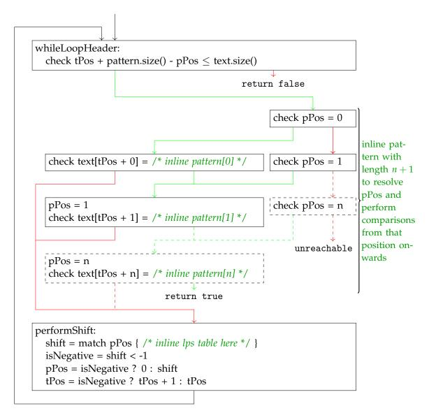
**Figure 3.2.:** General control flow of the generated code for the KMP algorithm with one loop. A green arrow is taken if the previous check evaluates to true, the red arrow otherwise.
