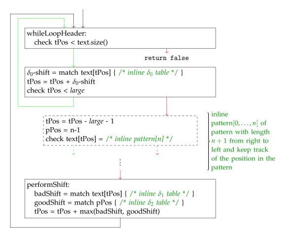
**Figure 3.5.:** General control flow of the generated code for the Fast BM. A green arrow is taken if the previous check evaluates to true, the red arrow otherwise.
