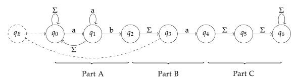
**Figure 5.3.:** Extended Like-NFA for pattern  $ab_a_%$ . The state  $q_B$  and dashed edges are inserted during the code generation process to handle backtracking.
