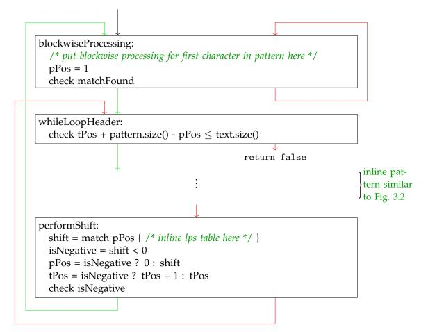
**Figure 3.3.:** Modified control flow of the generated code for the KMP algorithm with one loop to include optimizations. A green arrow is taken if the previous check evaluates to true, the red arrow otherwise.
