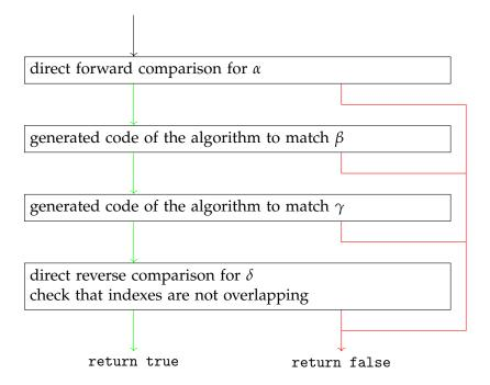
**Figure 3.6.:** Conceptual control flow of the generated code for the pattern  $\alpha \% \beta \% \gamma \% \delta$ . Each node encapsulates the whole functionality noted down in it. A green arrow is taken if the previous check or algorithm evaluates to true, the red arrow otherwise.
