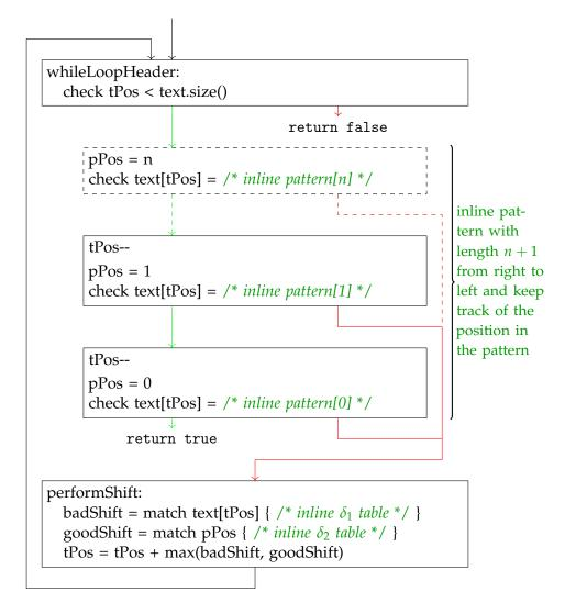
**Figure 3.4.:** General control flow of the generated code for the Original BM. A green arrow is taken if the previous check evaluates to true, the red arrow otherwise.
