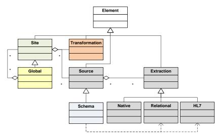
Figure 7.1: UML class diagram of the data architecture
