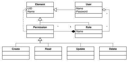
Figure 7.2: UML class diagram of the permission model
