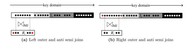
Figure 4.15: Outer and anti semi join processing require attention during the join phase: due to interpolation search and early stop of merge join the red tuples are skipped by inner MPSM
