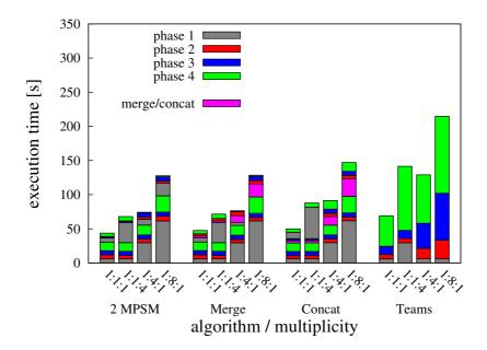
Figure 4.29: Performance comparison of two subsequent MPSM joins without postprocessing the intermediate result (2 MPSM), with merging each worker's intermediate result runs (Merge), and with concatenating the intermediate result runs (Concat)
