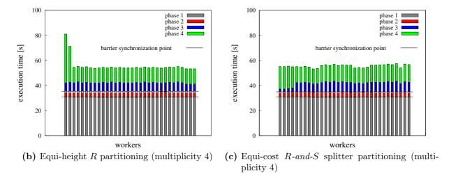
Figure 4.25: Effect of balancing splitters on MPSM performance
