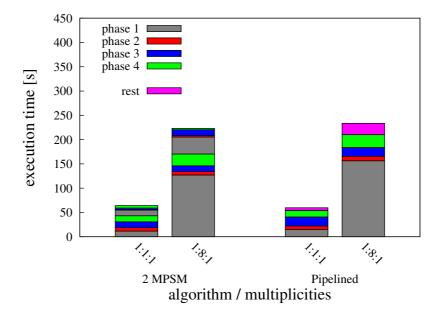
Figure 4.30: Performance comparison of two subsequent MPSM joins without postprocessing the intermediate result (2 MPSM) and pipelined MPSM (16 threads)
