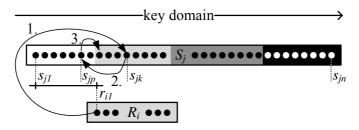
**Figure 4.10:** Interpolation search for  $r_{i1}$  in  $S_j$
