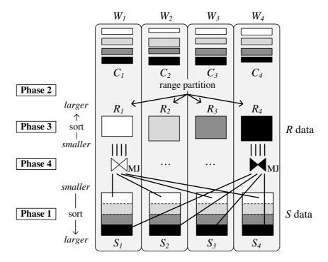
**Figure 4.6:** P-MPSM join with four workers  $W_i$
