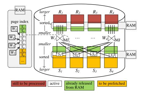
Figure 4.5: Disk-enabled MPSM join: the four workers  $W_i$  progress synchronously through their  $R_i$  run and all S runs, thereby only active parts of the runs are in RAM
