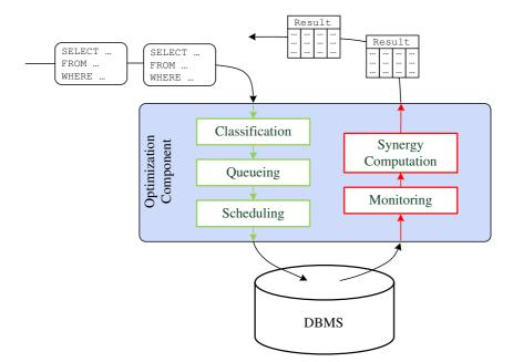
Figure 2.2: Architecture of the optimization component
